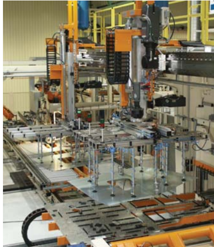
Conti laser welding systems, gantry handling and blank turning robot
