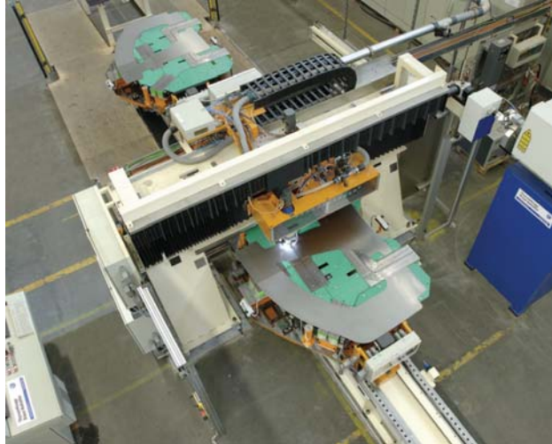
Gantry laser welding system, linear and non-linear weld seams, manual handling
