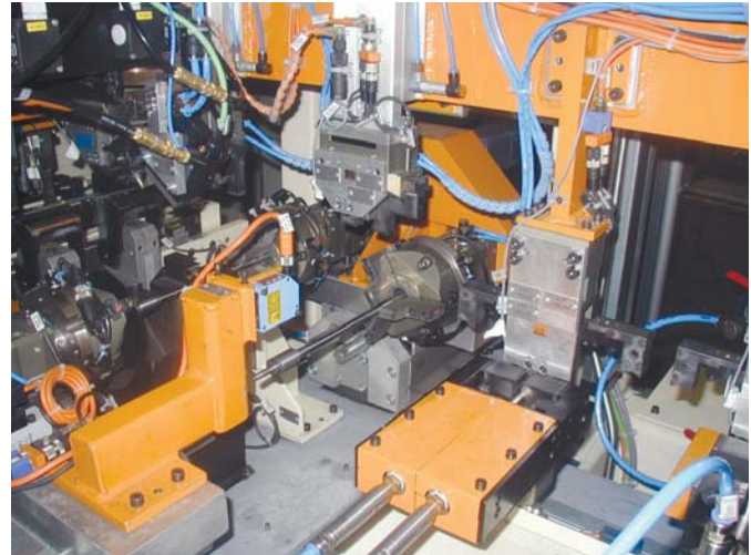
Laser welding system, joining and welding piston rods
