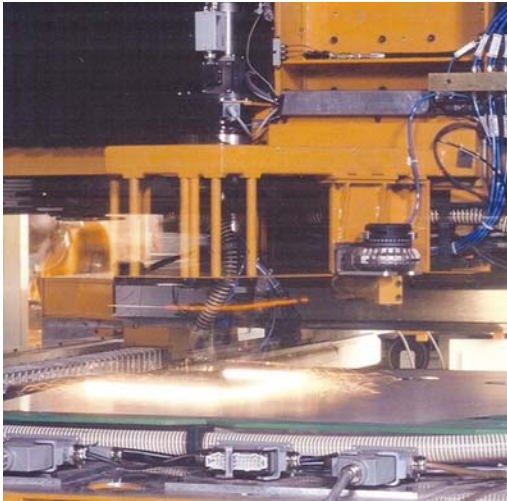
Gantry laser welding system, linear and non-linear weld seams, robot handling
